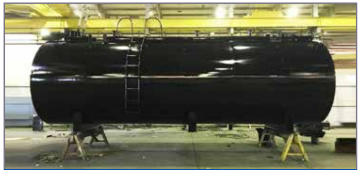
60 TON BITUMEN STORAGE TANK
